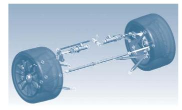
Engineers at Maserati and Dallara use MDO to simulate real-world forces on this Maserati MC12 race car suspension, reducing the number of physical prototypes and shortening the design cycle.
