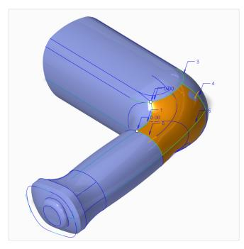
Advanced surfacing tools inside PTC Creo ISDX allow for the creation of high quality surfaces when more than 4 boundaries exist.
