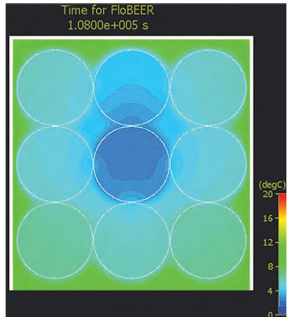
There's a bit of a cold bias towards the rear of the fridge, away from the door so either the bottom middle or bottom rear beer would be the best to grab first. Remember to move the remaining cans to fill the hole you've just left and turn either to the envelope or FloTHERM if you want to estimate or simulate (respectively) how long you should take to drink the current one until the next one has cooled further down to acceptable levels.
