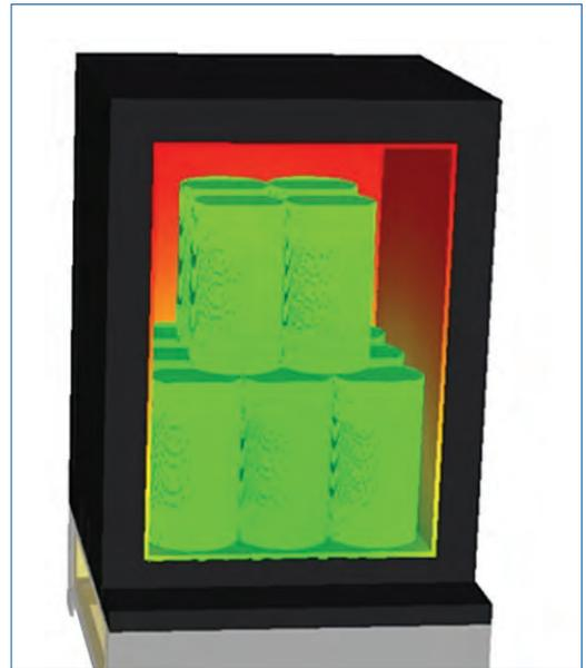
Compared to the average temperature of about 18 degC when the fridge was empty, the average temp when the beer's in the fridge has gone down to 13.6 degC with the average temperature of the beer itself down at 10.1 degC. Not all cans are equal, not surprisingly the can sitting on top of the cold plate is coldest (shown here by hiding the 3 cans at the front):
