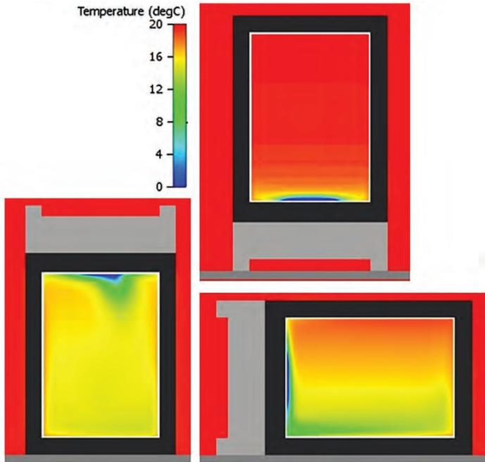
The mixing effects of the cold dumping air can be seen when you start to animate the airflow inside the fridge (note I've reduced the temperature range to go from 14 to 16 degC, blue is  $\leq 14$ , red is  $\geq 16$  to clearly show the hot air (rising) and the cold air (sinking), note that the speeds are not to 'scale'):
