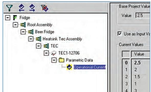
One click of the GO button will have FloTHERM solve all these variants and present the results back. One of the simplest ways to inspect the results is to note 'monitor point' temperatures, temperatures at defined points in the model, in this case inside the fridge right at the bottom, in the middle and at the top:
