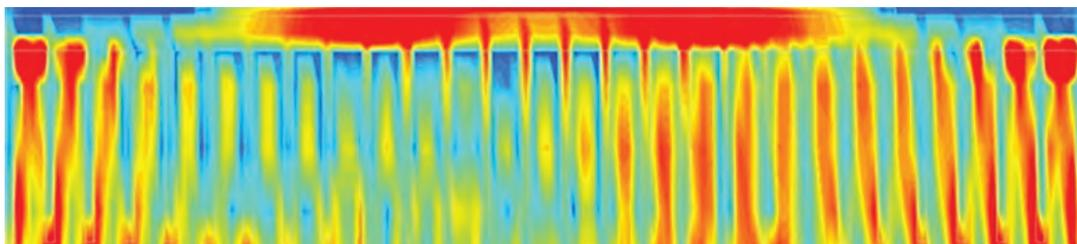
To relieve a bottleneck you could use a material with a higher thermal conductivity, or make the cross sectional area the heat passes through, larger. The latter is much cheaper, let's increase the base thickness in the middle portion some more:
