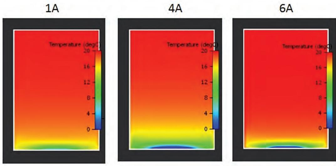
Due to our friend 'stable stratification' even the colder air at 4A at the bottom of the fridge is just sitting there. There is no way for the cold to reach up to the top of the fridge. So in all cases the top of the fridge remains too warm (unless you're a real ale drinker).
