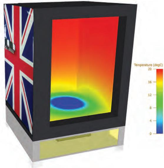
The Union Jack was simply a matter of using FloTHERM's texture mapping capability, using a JPEG image taken by my phone camera. A 'fly-by' animation can be created by setting a few choice view points locations which are then traversed in sequence and output as an .avi (I used Corel™ to convert to an animated GIF). This, and all subsequent animation sequences, can be viewed in the original blog postings at <http://blogs.mentor.com/robinbornoff/>
