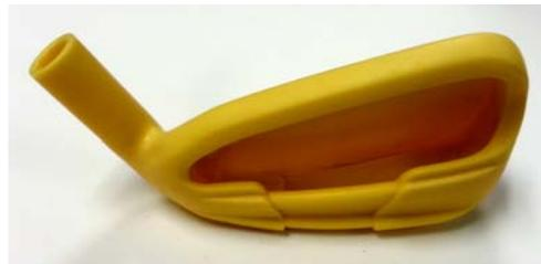
Nivanh uses the ULTRA DLP along with two other printers to complete rapid prototyping of club heads. According to Nivanh, the company began using 3D printing to cut production costs, but their Objet printer was not allowing them to complete tasks efficiently. Nivanh sends the builds to a vendor who then makes the final cast. They use Siemens PLM NX, a CAD/CAM software solution, to design the prototype before running the file through Magics to print.
