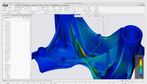
Creo includes tools for finite element analysis, computational fluid dynamics, and more.
