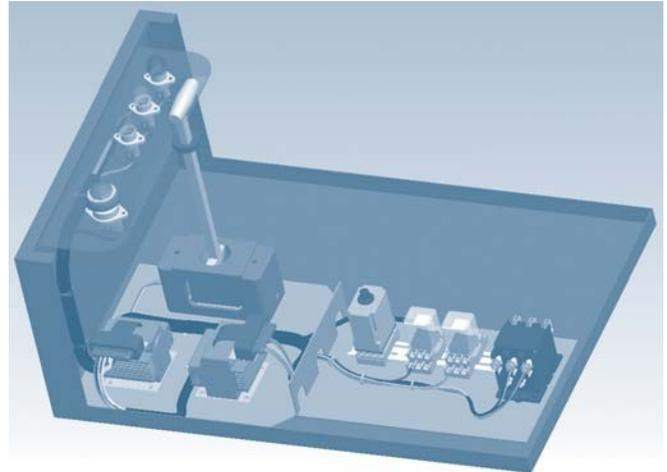
With Pro/ENGINEER Cabling Design, you can automatically route cables within your model, ensuring a fully defined digital model.
