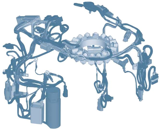
Engineers at Bombardier Recreational Products used Pro/ENGINEER Cabling Design to design this wire harness. Pro/ENGINEER Cabling Design makes it easy to move components and connectors without manually re-routing wires and cables.
